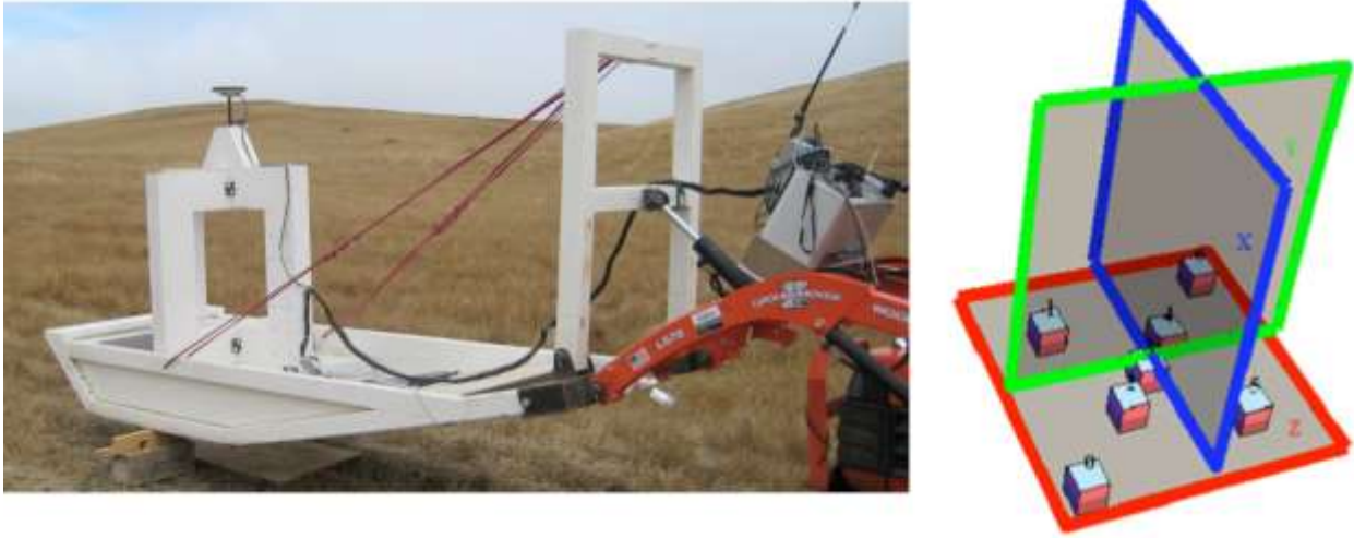
Figure 3.1: The MetalMapper during SLO site deployment (left) and its schematic diagram (right).
