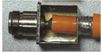
Fig. 70. Cable termination with adapter and N-type connector
