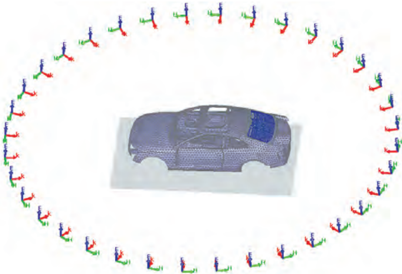
Fig. 29. Car body exposed to plane waves incident from different angles
