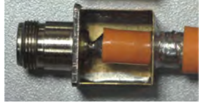
Fig. 78. Cable termination with adapter and N-type connector
