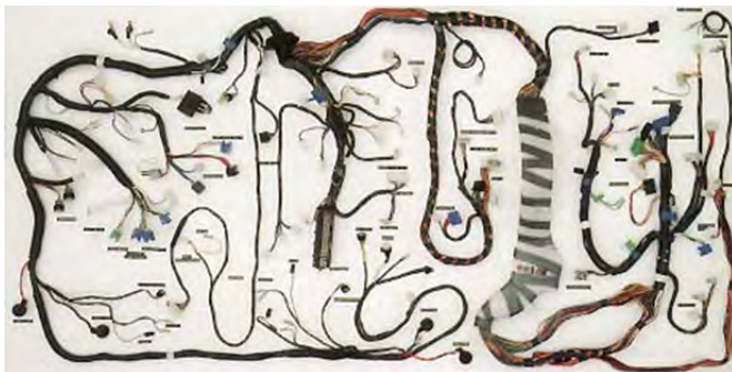
Fig. 36. Part of the cable harness of an automobile
